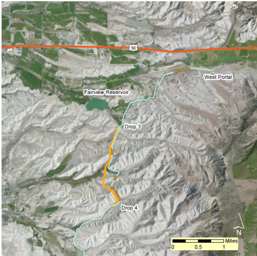
Figure 3. The yellow line indicates the proposed alignment of the new overhead power line. The blue line represents the location of the South Canal, with brown indicating where the canal is tunneled through the adobe hills.
